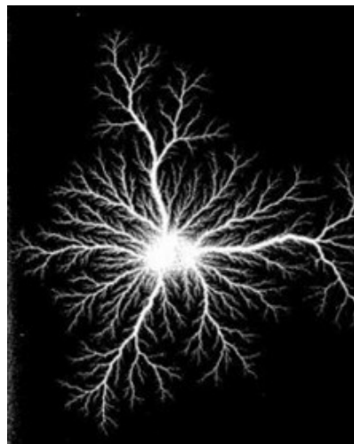
Figure 9: FL in tetra-fluoride gas under 30kV voltage and 30.3atm pressure (Pereira et al. [2021]).
