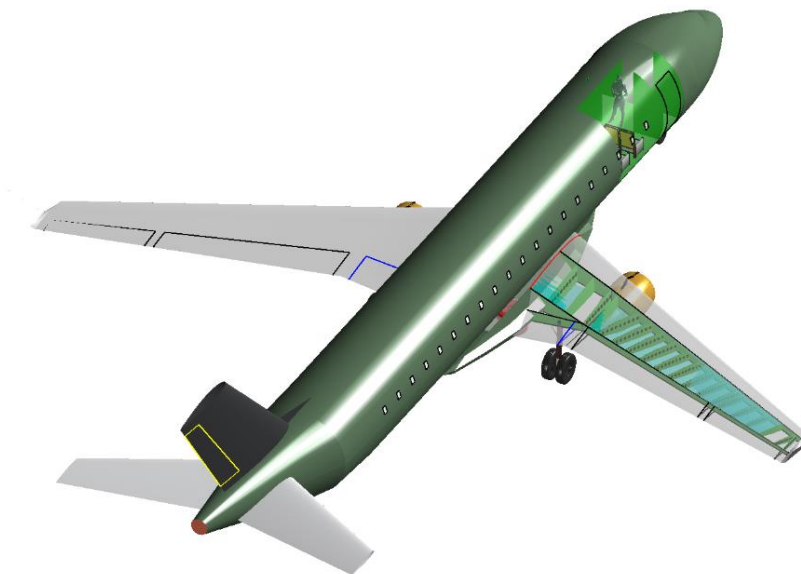
Figure 17: Example of wing layout for a 72-passenger airliner fitted with underwing engines
