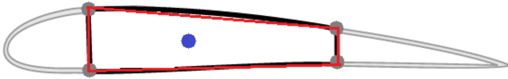
Figure 19: Approximation of the Wingbox Cross Section as an Isosceles Trapezium
