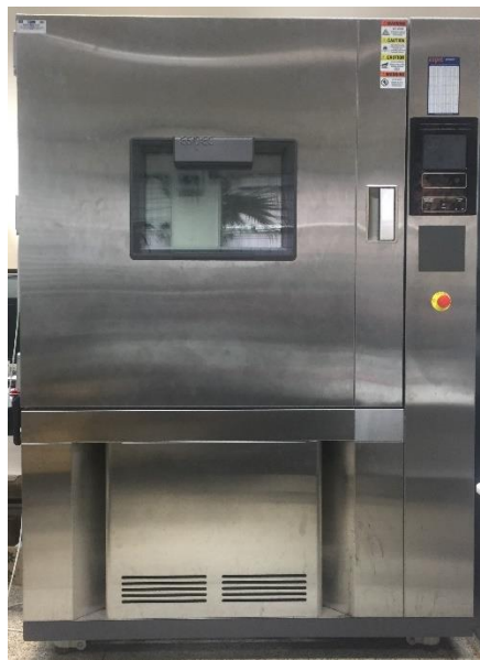
Figure 14: Platinous EPL-4H series climatic chamber used in this test.
