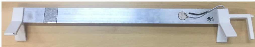
Figure 16: Specimen used in the test illustrating the PZT patch and damage position.
