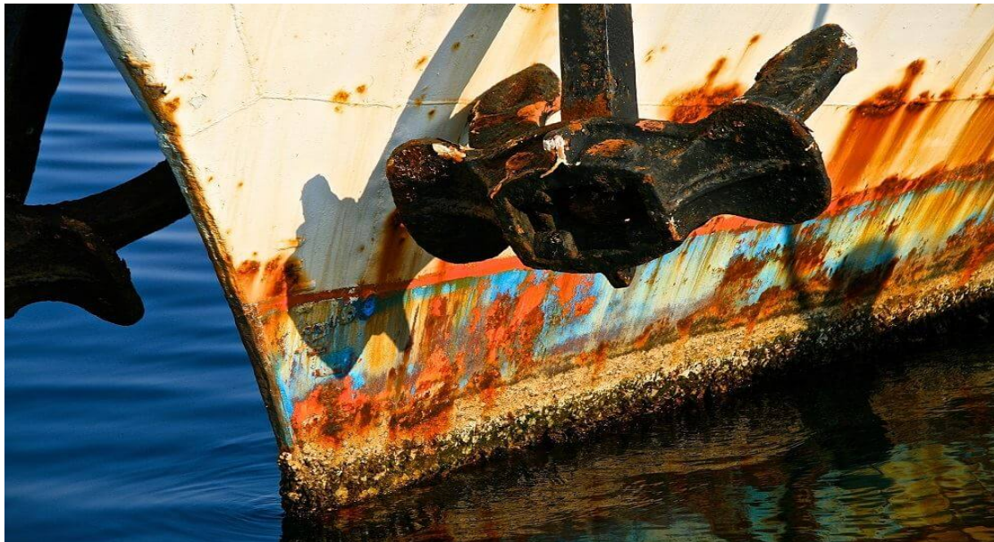
Figure 15: typical hull corrosion stages [25]
