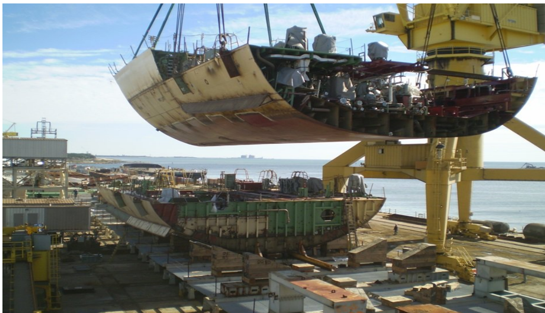
Figure 8: Ship modular construction in a shipyard [15]
