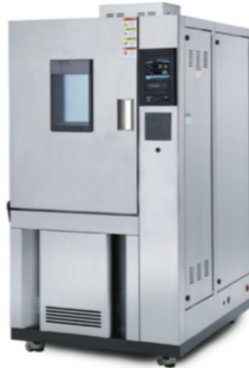
Figure 8: Climatic chamber used in the experiment. Source: Freitas et al. [2021c].
