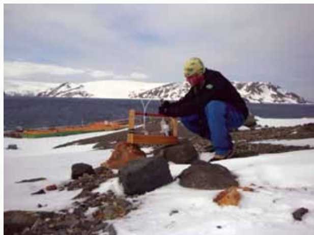
Figure 1. Collect the air samples using stainless steel cylinders with electropolishing internal pressurized to 2 atm, near (left, on the beach) and far from the station (right).
