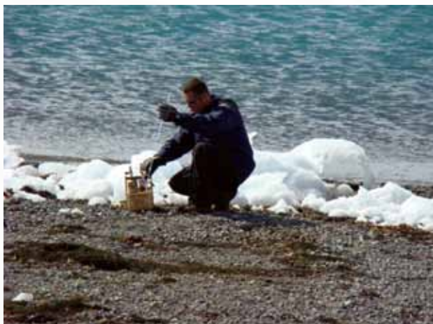
Figure 1. Collect the air samples using stainless steel cylinders with electropolishing internal pressurized to 2 atm, near (left, on the beach) and far from the station (right).
