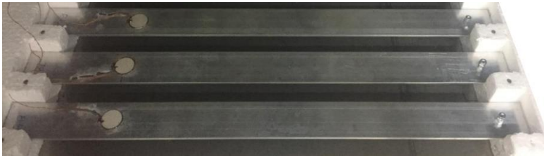
a) Structural Systems (Aluminum Beams + PZTs Insert).
