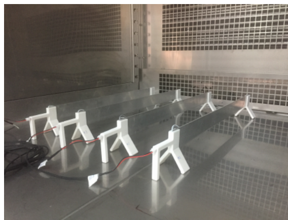
Figure 10: Positioning the specimens inside the chamber. Source: Freitas et al. [2021c].
