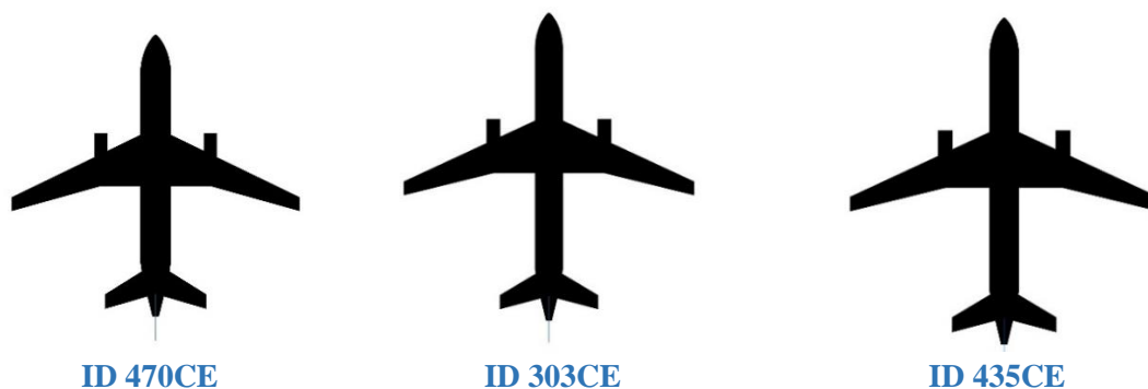
Figure 29: Top view of some individuals in the Pareto front of classic design simulation (not on the same scale)
