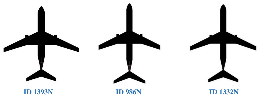
Figure 25: Top view of some individuals in the Pareto front of niche design simulation (not on the same scale)
