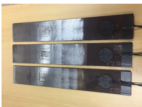
a: Specimens instrumented with PZT patches.
