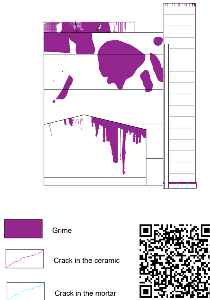
Figure 13 – Damage map of the left side façade
