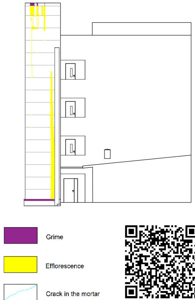
Figure 15 – Damage map of the right-side façade
