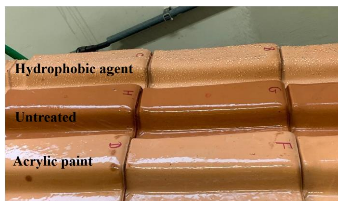
Figure 6 - Behavior of clay roofing substrates with different treatments.
