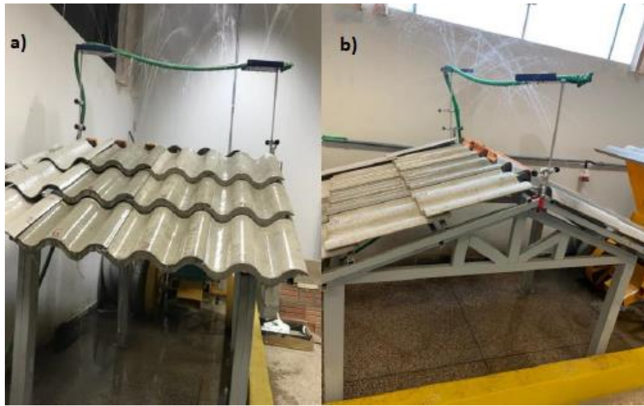
Figure 5 - Roofing substrates exposed to the rain simulator: a) Lateral view of the roof; b) Front view of the roof.
