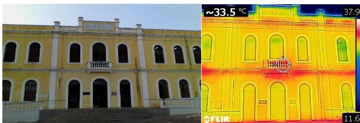
Figure 18 - Thermographic map of the Vale do Acaraú State University (UVA) - Betânia Campus façade in the afternoon.
