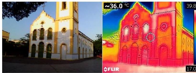
Figure 5 - Thermographic map of Church of Sorrows in the afternoon.
