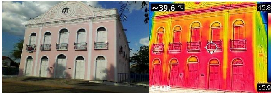
Figure 2 - Thermographic map of the facade of São João Theater in the afternoon.
