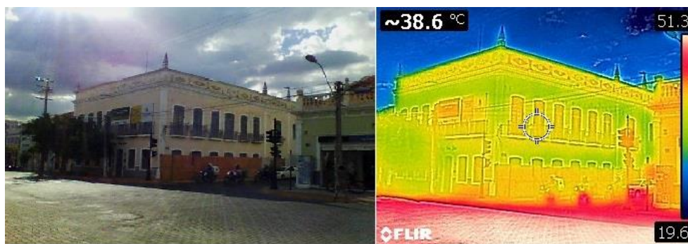
Figure 14 - Thermographic map of the facade of the Dom José Museum in the afternoon.
