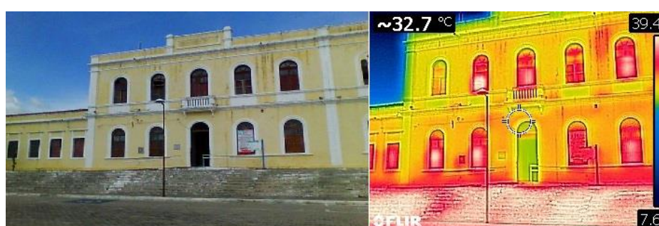
Figure 20 - Thermographic map of the Vale do Acaraú State University (UVA) - Betânia Campus facade in the morning at the secondary entrance.
