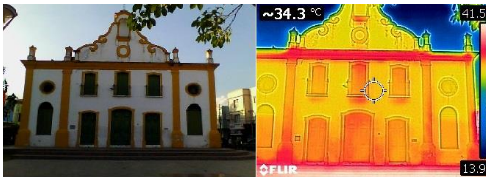
Figure 11 - Thermographic map of the facade of Church of the Rosary in the afternoon.
